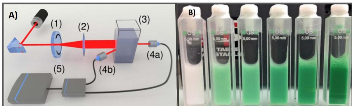
**A** – Set-up of the automated determination of  $l^*$  and absorption. Both, the transmission (4a) and the backscattering (4b) intensity of the sample (3) is measured. In order to allow measurements on non-ergodic samples, the incoming laser beam is scrambled by a rotating ground glass (1).
